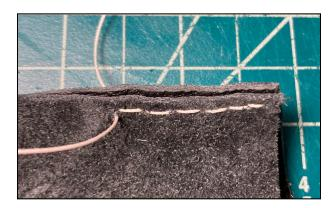
Figure 6: a saddle stitch moving along the seam from the top of the shoe (on the right) toward the bottom (on the left).
