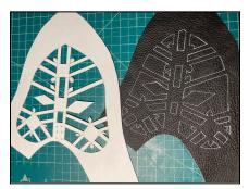
Figure 2: the template and its tracing in white gel pen on the leather upper. (The small nodules will be more completely defined by carefully cutting away the leather at their bases.)
