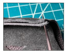
Figure 5: the first hole on the side seam - the leather is grain to grain (smooth sides together) and these edges will project into the shoe.
