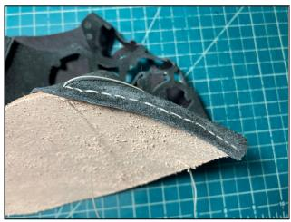
Figure 8: a run of saddle stitches from the toe along one side of the shoe.
