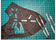
Figure 3: a variety of X-Acto knife blades facilitates cutting the leather: curved blades are best for long lines; short angled ones work well for shorter lines; a square blade is best on corners and delicate parts.
