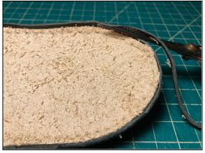
Figure 10: trimming away excess upper, the last step before soaking and turning the shoe.
