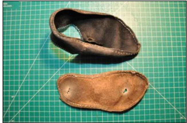
*Shoes with worn-out soles (left) and a detached upper/sole (right).*
