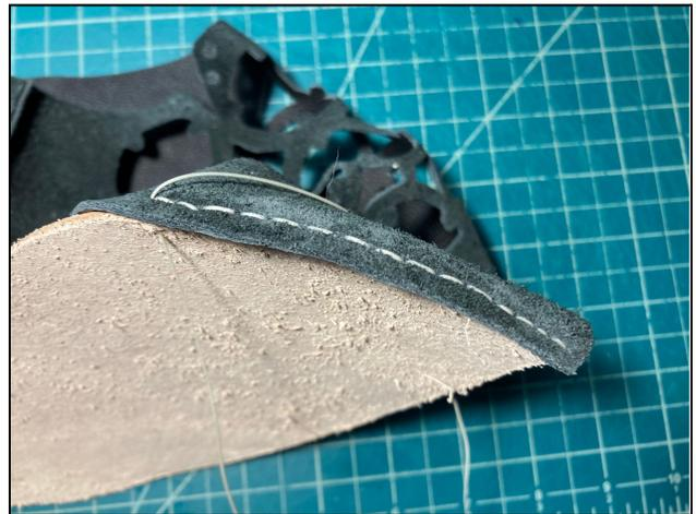
Figure 8: a run of saddle stitches from the toe along one side of the shoe.
