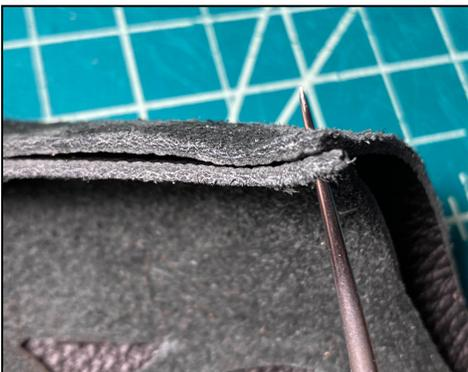
Figure 5: the first hole on the side seam - the leather is grain to grain (smooth sides together) and these edges will project into the shoe.
