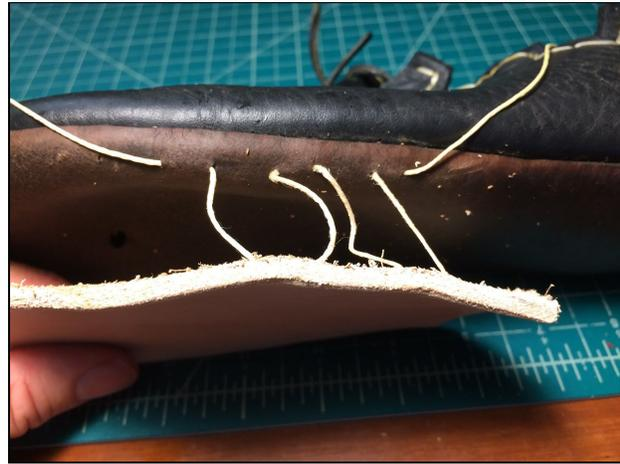
*First tunnel being made with awl in old sole (left) and several tunnels in old and new soles (right).*
